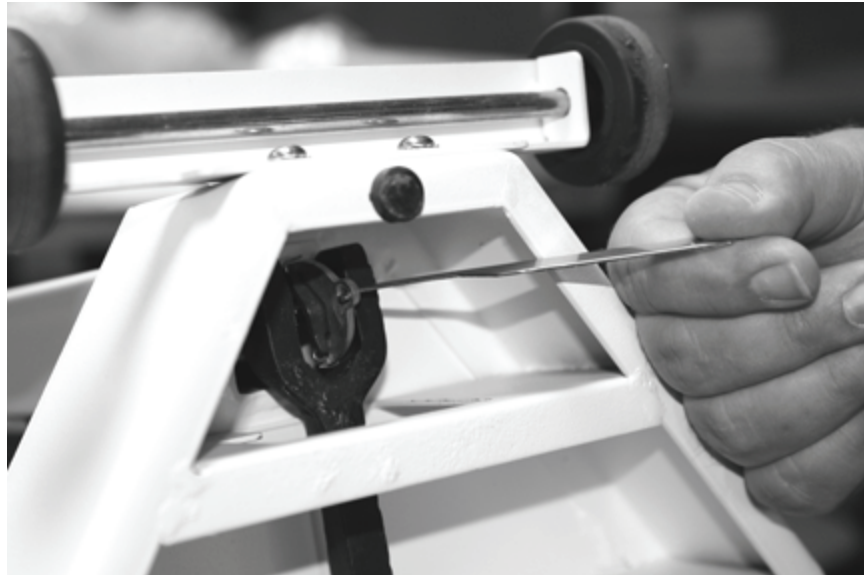
Figure 5. Connecting the Steelyard Rod to the Scale Base
