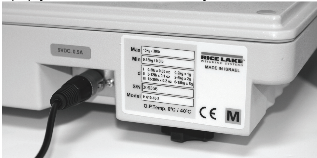
Figure 3. AC Power Connection Site
