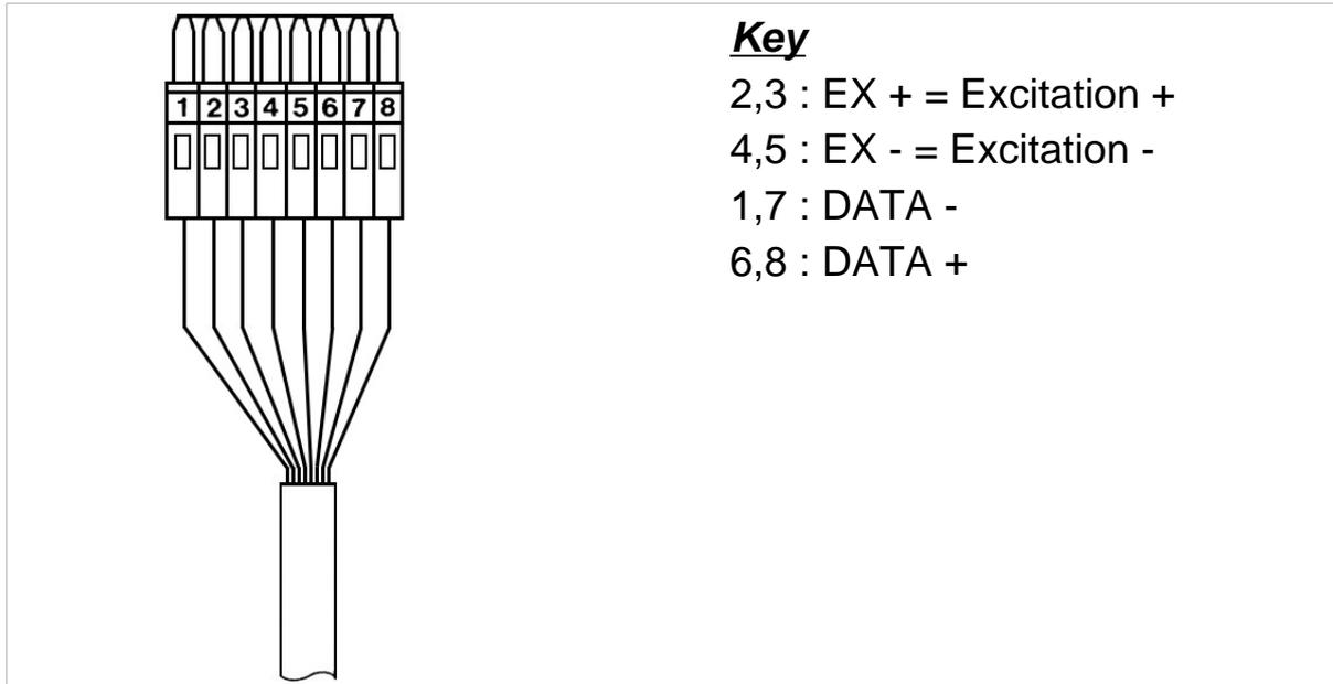
**Figure 3.7 - Pinout of JBILDGT connector for connection to scales with digital load cells** (*citi0609.gif*)
