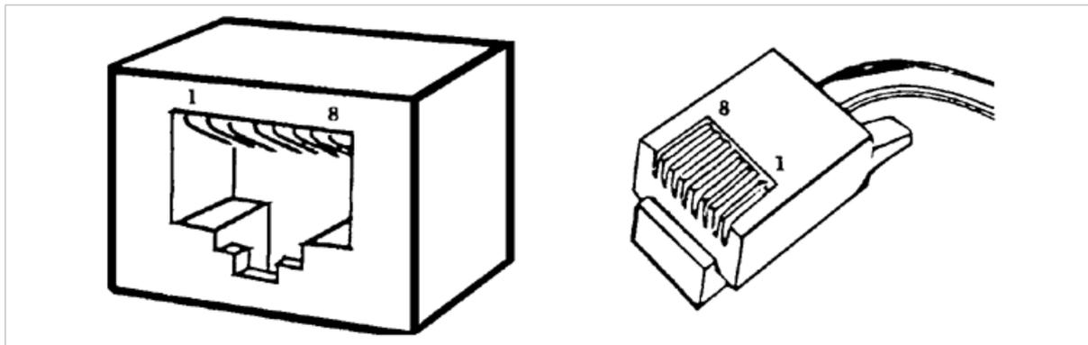
**Figure 6.10 - Pin numbering for RJ-45 8-pin connector (log0066.gif)**
