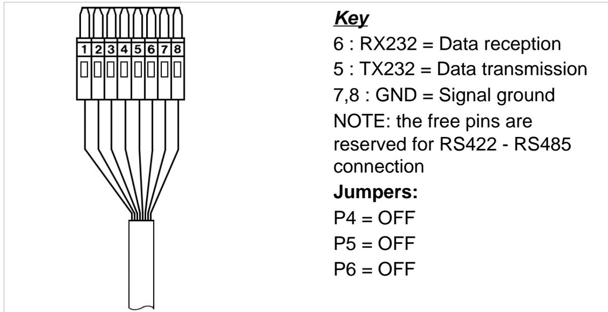
**Figure 3.10 - COM2 serial port connector (8-pin)** (*citi0609.gif*)
