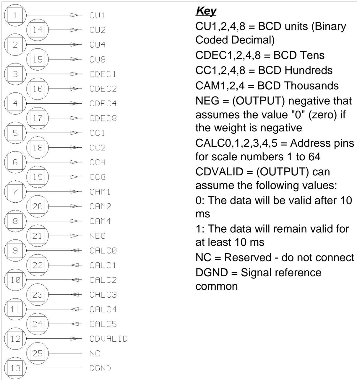
**Figure 6.4 - Calculator BCD output connector (log0061.gif)**
