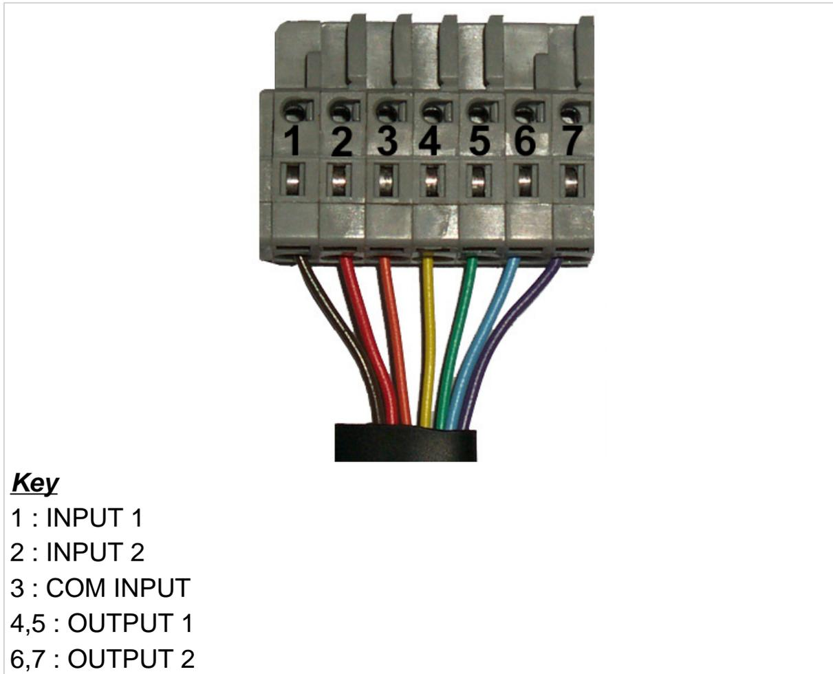
**Figure 3.14 - Input/output terminal board wiring diagram**
