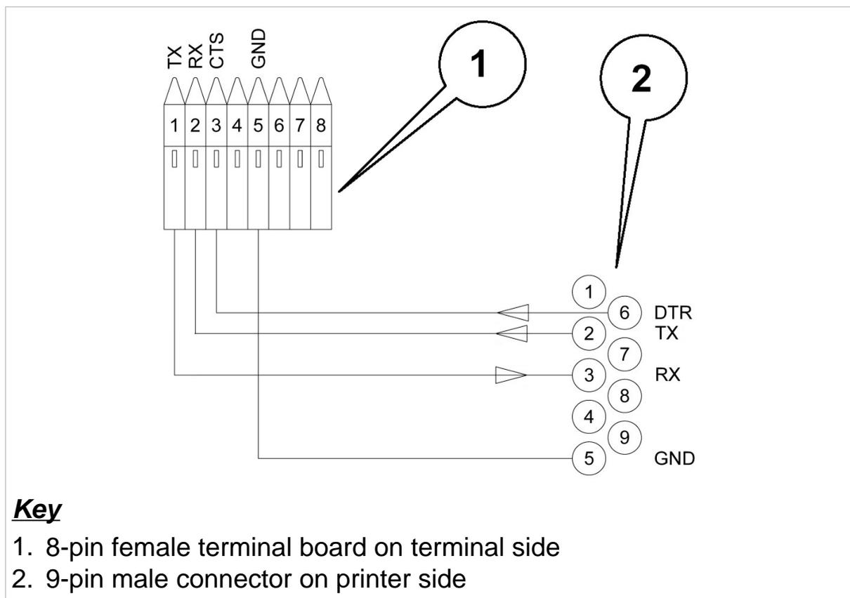
**Figure 6.12 - Connection with STB60 in the RS232 mode**
