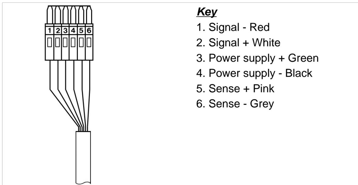
**Figure 3.6 - Pinout for the JCELA and JCELB connectors for connection to scales with analogue cells (*citi0608.gif*)**
