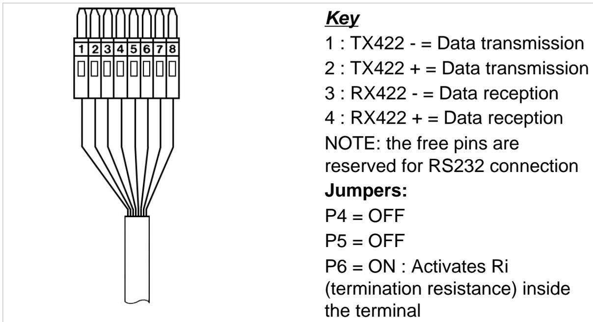
**Figure 3.11 - Example of RS422 serial port connection**(*citi0609.gif*)
