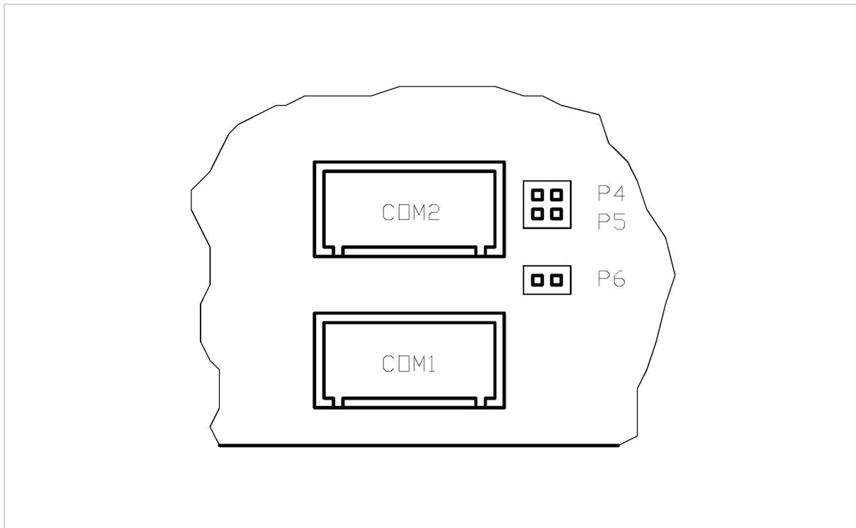
**Figure 3.9 - Positions of jumpers P4,P5,P6 on the CPU board**
