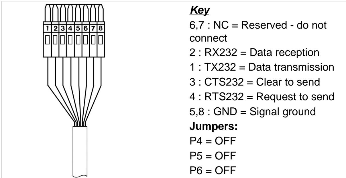
**Figure 3.8 - Standard serial port connector (8-pin) (citi0609.gif)**
