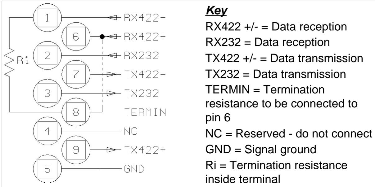
**Figure 6.8 -Supplementary serial port connector (9-pin female D-type) (log0064.gif)**
