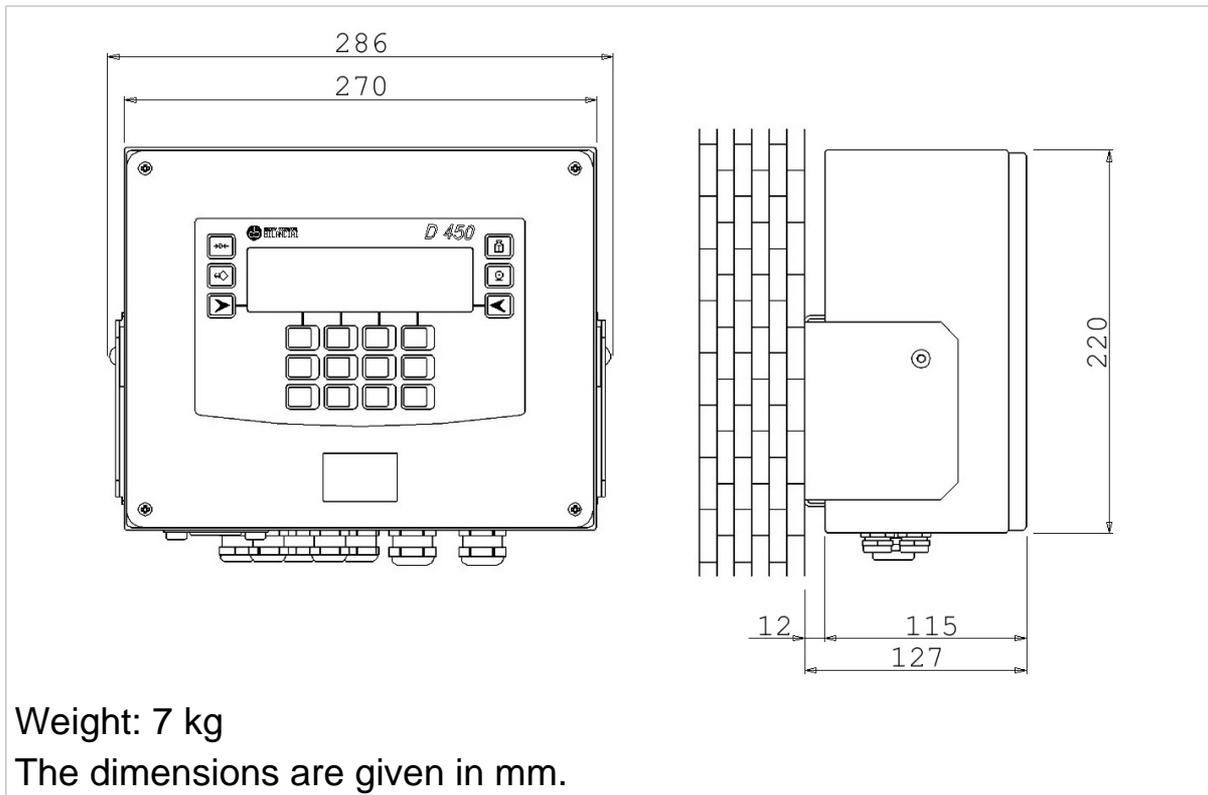
**Figure 1.1 - Dimensions and weight of the wall-mounted terminal version (citi0601.jpg)**
