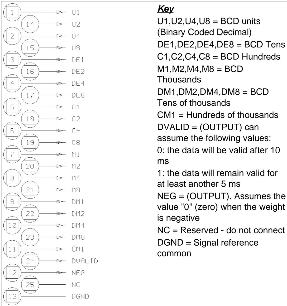
**Figure 6.3 - Parallel 5V TTL BCD output connector (log0060.gif)**
