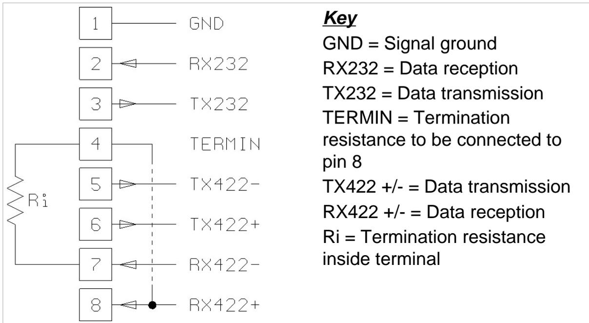
**Figure 6.9 - Supplementray serial port connector (RJ45 8-pin)(comx2) (log0065.gif)**
