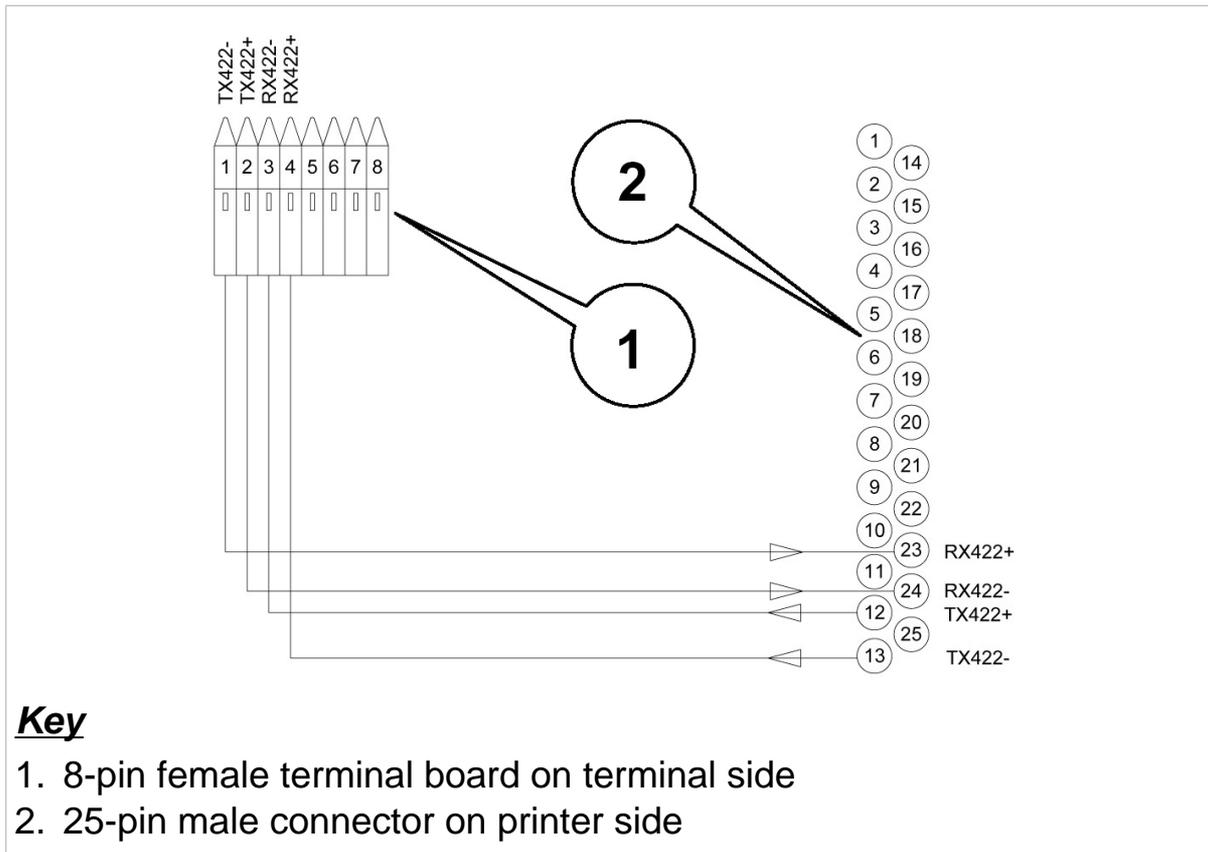
**Figure 6.14 - Connection with STB112 in the RS422 mode**
